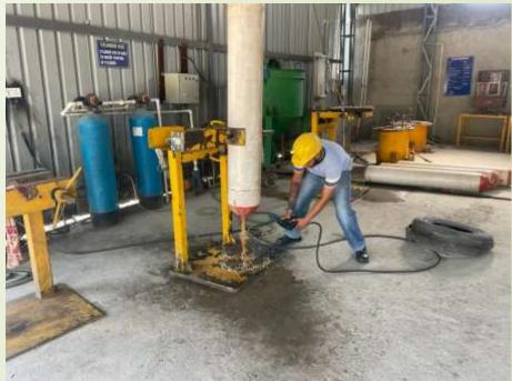
□ WEIGHING & INSPECTION (REJECTED IF LOSS IN TARE WT. IS MORE THAN 5%
